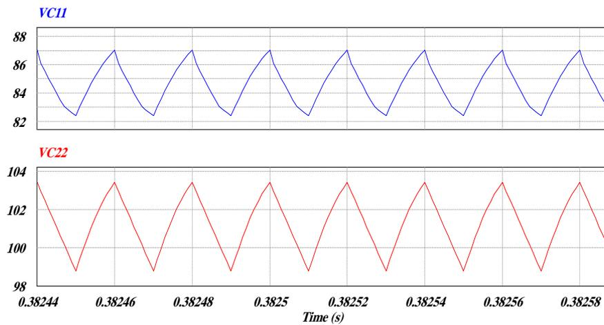
Figure 7. voltages across capacitances C11 and C22
