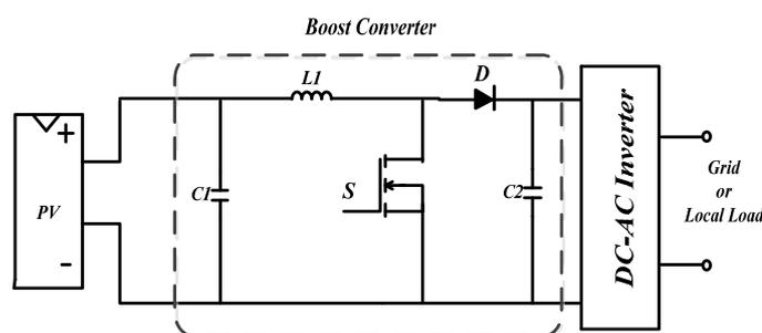
Figure 1. Diagram of Conventional PV power generation system
